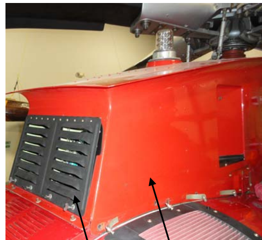
Figure 2-1. FILTER MAINTENANCE AID – (ABOVE) “YELLOW Indicator” position relative to SAFE OPERATING ZONE (“GREEN Zone”) or SERVICE FILTER (“RED Zone”) markings defines current filter condition and pushing “YELLOW RESET Button” resets indicator. NOTE: FMA units for both engines are located at the back of the rear upper cowling and may be read or reset via access door at the aft end of the cowling.
