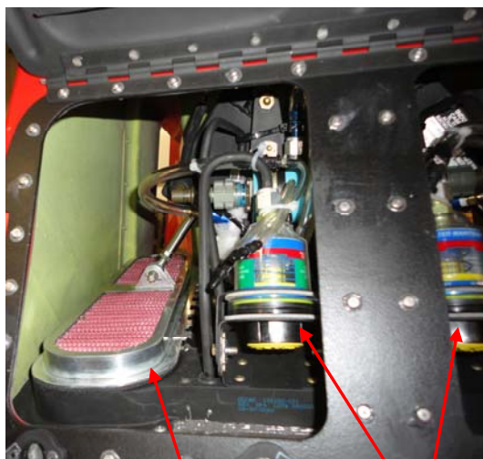
Figure 2-1. FILTER MAINTENANCE AID – (ABOVE) “YELLOW Indicator” position relative to SAFE OPERATING ZONE (“GREEN Zone”) or SERVICE FILTER (“RED Zone”) markings defines current filter condition and pushing “YELLOW RESET Button” resets indicator. NOTE: FMA units for both engines are located at the back of the rear upper cowling and may be read or reset via access door at the aft end of the cowling.
