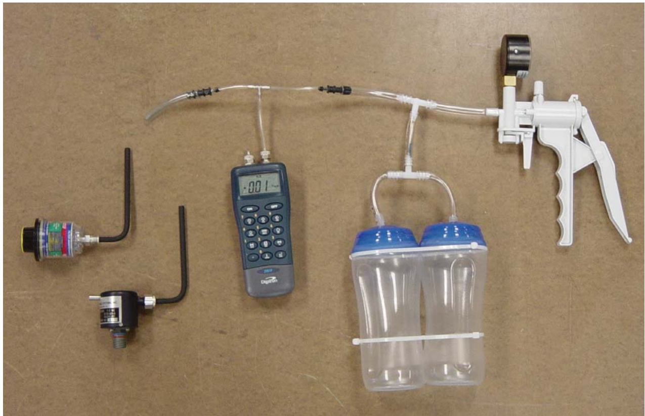
Picture 7: Test Setup with Manometer
