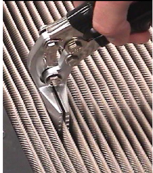
Picture 6: Hand Seamer Used to Straighten or Crimp Pleats
