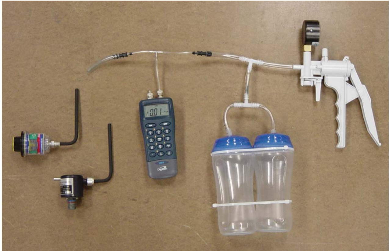
Picture 6: Test Setup with Manometer
