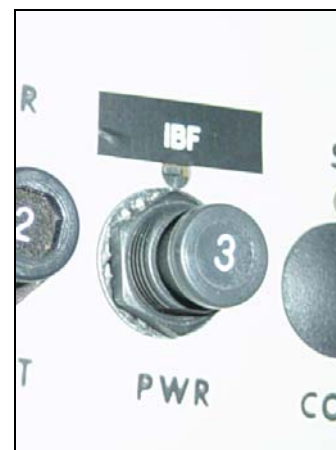
Picture 3: Circuit Breaker
