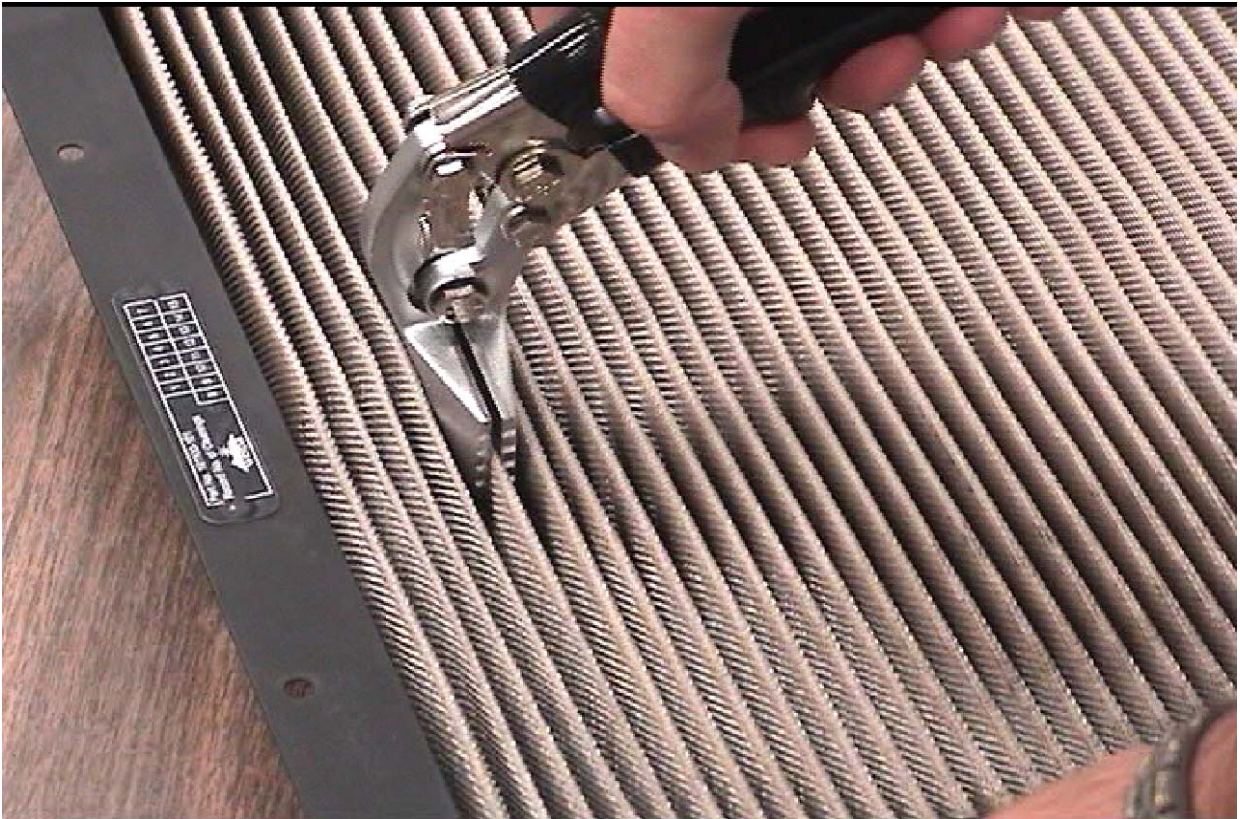
Figure 7: Hand Seamer used to Straighten or Crimp Pleats
