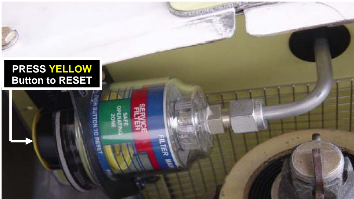
Picture 3-2: FMA RESET LOCATION - unit is mounted to bottom of IBF floor assembly and is accessed through RH access door on air induction cowling.
