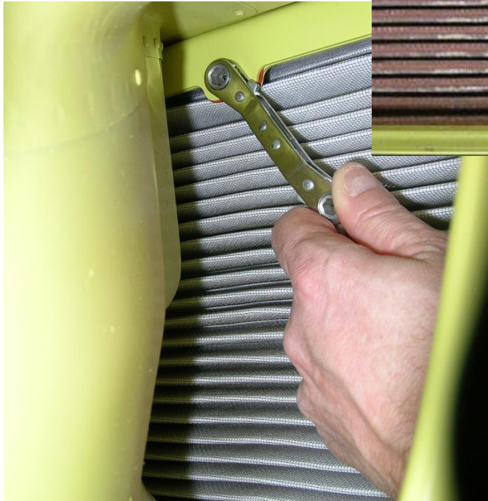
Picture 8-2: INSTALLATION/REMOVAL OF BOLTS SECURING FILTER ASSEMBLIES TO FILTER ADAPTER FRAME
