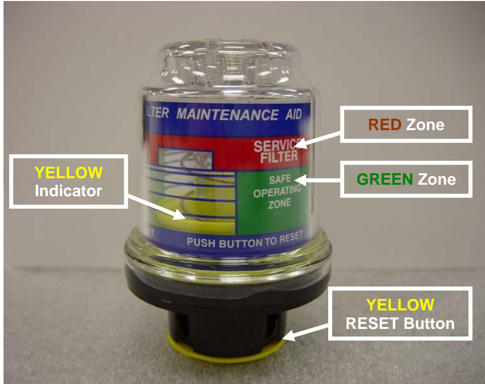
Figure 2-1. FILTER MAINTENANCE AID – (ABOVE) “YELLOW Indicator” position relative to SAFE OPERATING ZONE (“GREEN Zone”) or SERVICE FILTER (“RED Zone”) markings defines current filter condition and pushing “YELLOW RESET Button” resets indicator. (BELOW) FMA unit is mounted on the outside of the inlet cowling and can be viewed by opening the inspection door.
