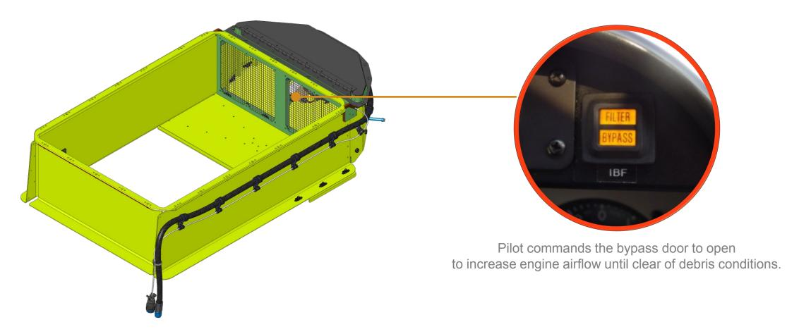
**NOTE:** Aircraft with particle separators must land immediately during heavy debris conditions and do not have the ability to keep flying like aircraft with a barrier filter bypass system.
