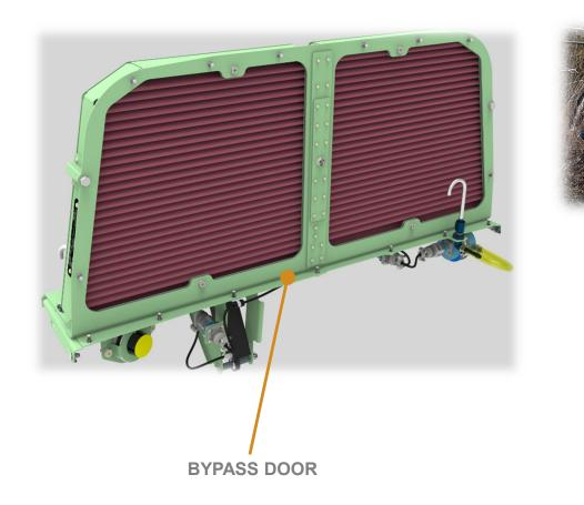
Pilot commands the bypass door to open to increase engine airflow until clear of debris conditions.
