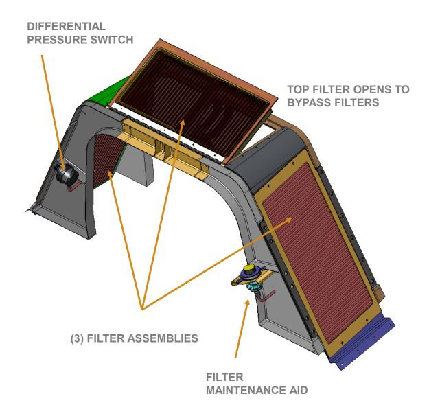
THE DONALDSON IBF SYSTEM REPLACES THE CURRENT INTAKE SCREEN AND INTAKE FARING ASSEMBLY WITH A NEW IBF ASSEMBLY
