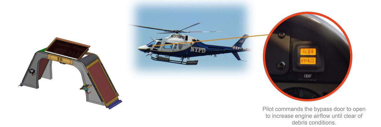
**NOTE:** Aircraft with particle separators must land immediately during heavy debris conditions and do not have the ability to keep flying like aircraft with a barrier filter bypass system.
