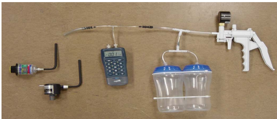
Figure 8-3: EXAMPLE OF TEST SETUP WITH MANOMETER
