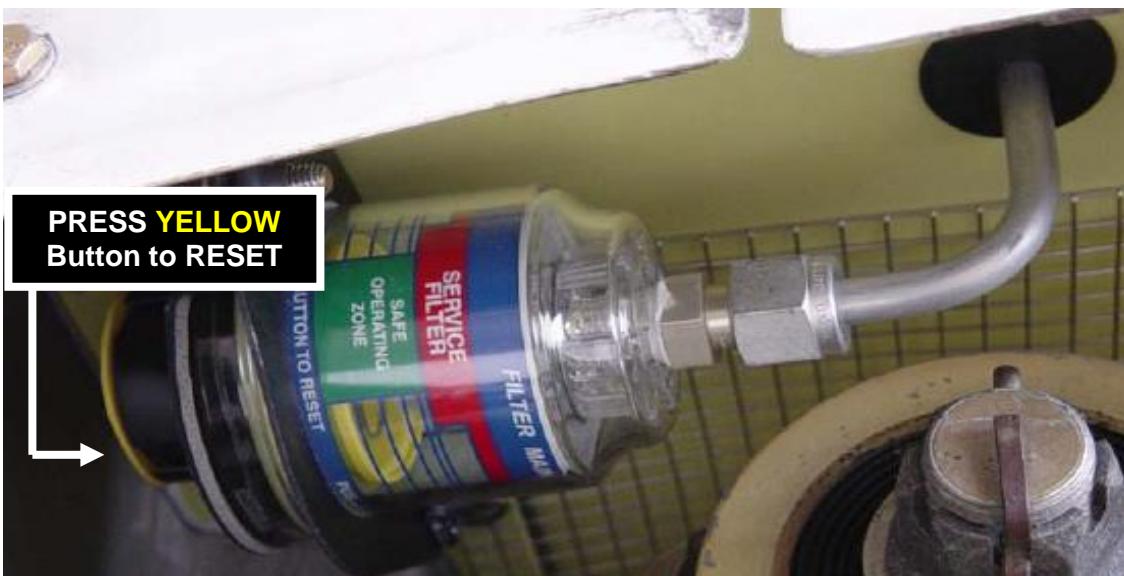
Figure 3: FILTER MAINTENANCE AID
