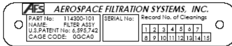
Figure 3: EXAMPLE OF FILTER ASSEMBLY DATA PLATE
